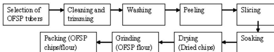
**Fig. 1: Flow chart of OFSP dried chips and flour production**
